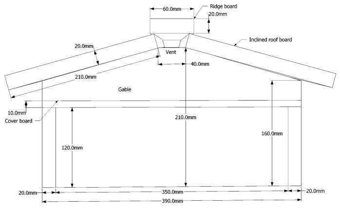
If thinner wood is used for the inclined boards, they may be nailed to the ridge board from their undersides by supporting the three pieces inverted with blocks suitably positioned to give approximately the correct angle. The unit of three boards is then nailed on to the gables.
