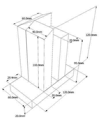
The leg has a wide foot attached to prevent the hive from sinking into the ground and possibly toppling. Furthermore it gives a 20-30 mm projection outside the footprint of the floor, thus greatly increasing stability.
