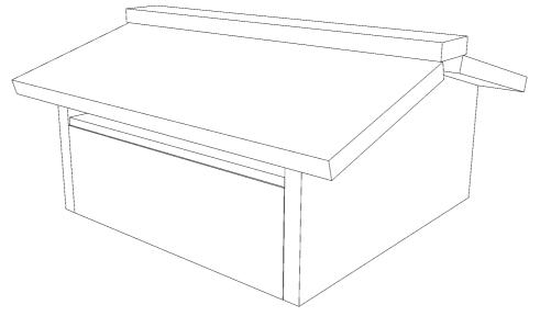
The example given here uses 20 mm wood for the outer structure. This is based on Warré's plans. Wood of 15 mm thickness would be perfectly adequate and make for a lighter roof. There is 10 mm play between the roof inner walls and the quilt outer walls to ease placement and removal of the roof.
