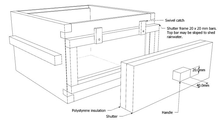
This design places the insulation flush against the glass, the depth of the cavity exactly matching the depth of the shutter. To minimise jamming of the shutter in wet conditions, it may be made one or two millimetres smaller in each direction.
