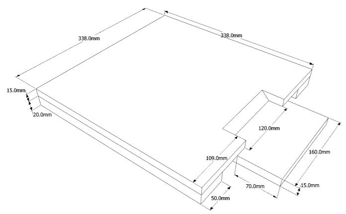
Warré recommended 15-20 mm for the thickness of the floor. He gave no guidance on the thickness of the battens underneath it.
