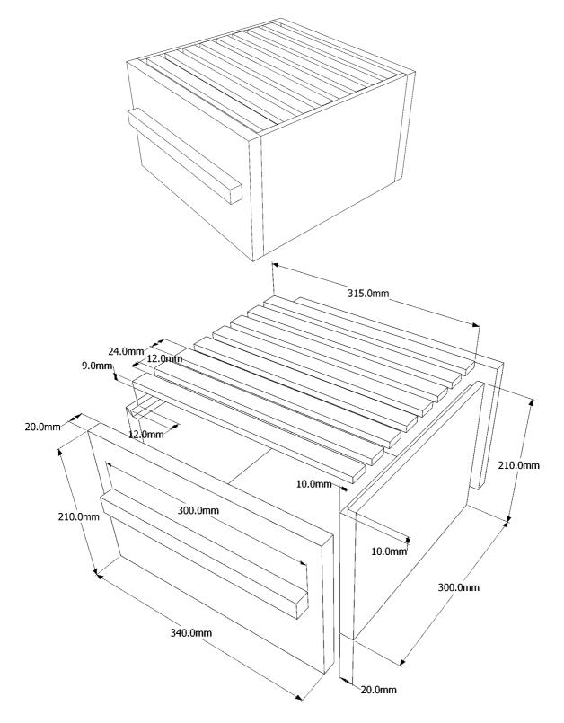
The spacing between all bars and between the end bars and the walls is 12 mm. The rebates can be cut with a table saw, a rebating plane or even with a hand saw provided that a guide is affixed to the wood first. Warré specifies a top-bar length of 315 mm. If it is extended close to 320 mm, then it better spans the rebate and leaves no cavity for pests to occupy.
