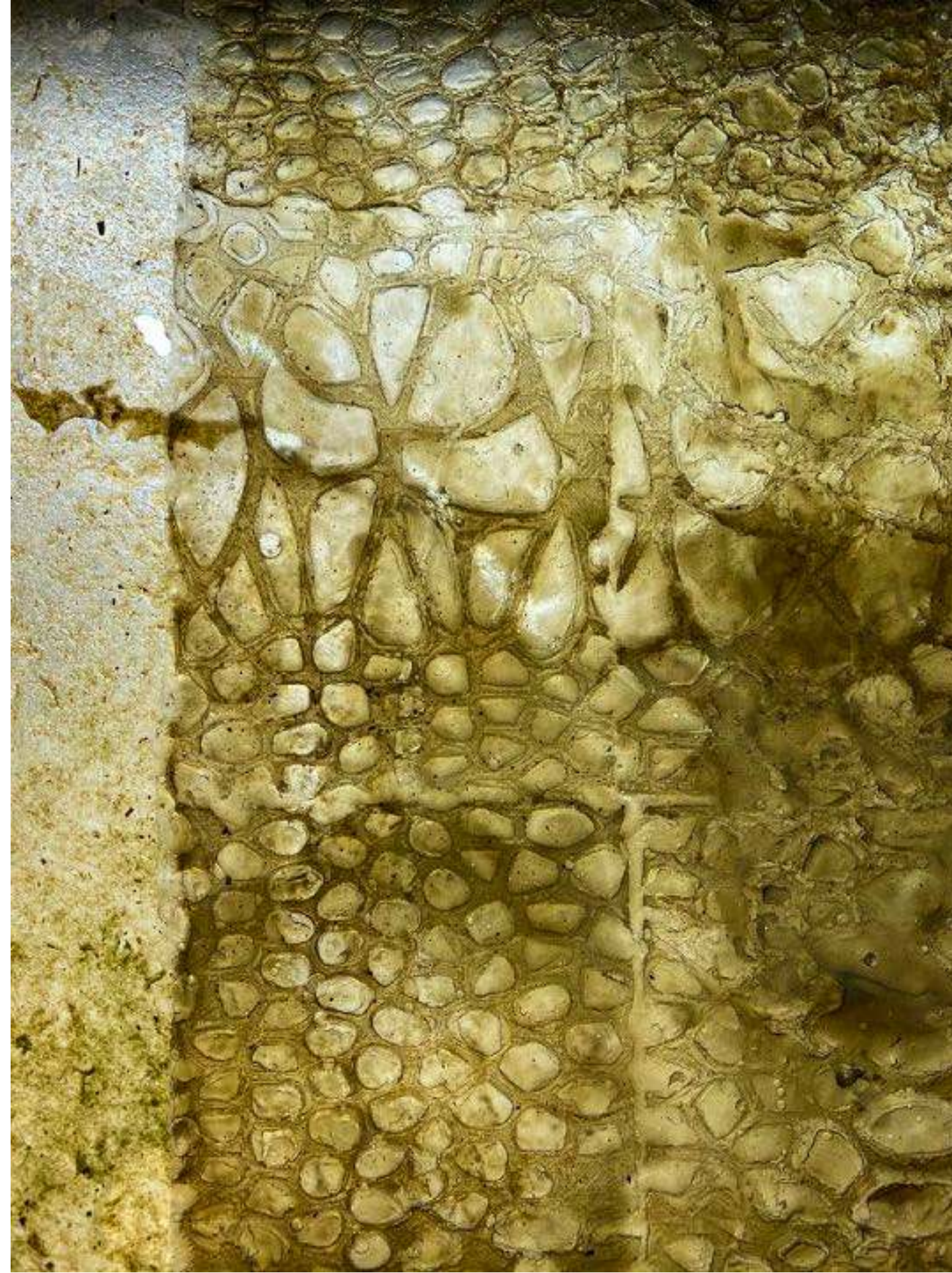
above: biotextile on basis of agar agar and with natural pigments. The design is created in a mould made from 3D printed designs. right: red algae woven work
