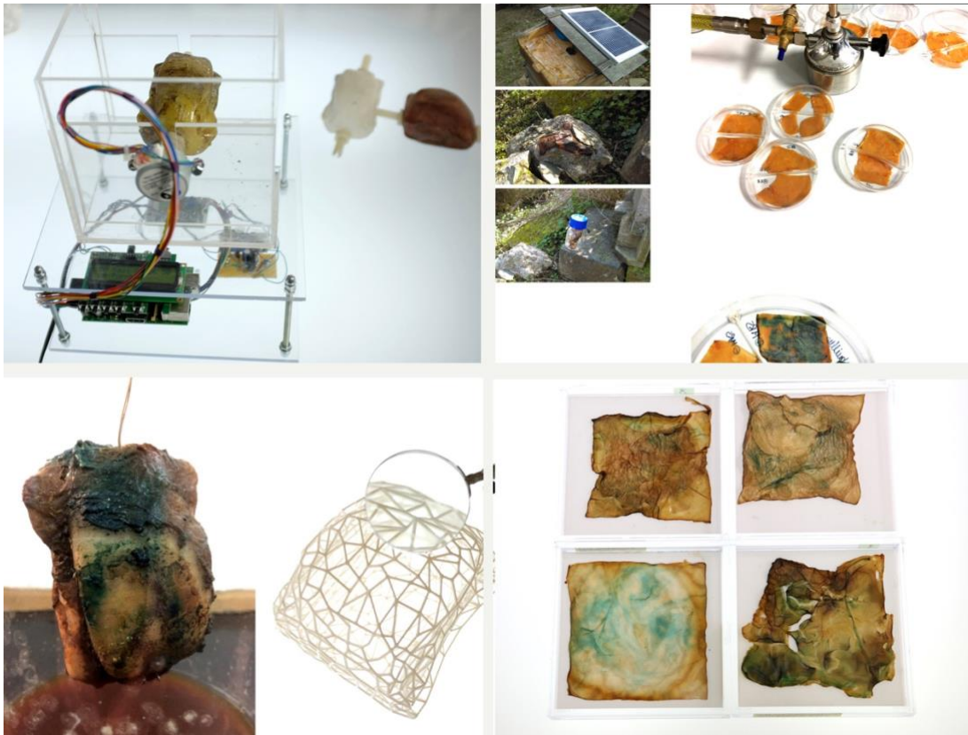
Figure 5. Clockwise from left to right: growing cellulose skin on a rotating object; bacteria hunting in the forest, Lactobacillus plantarum on dry cellulose skin; Lactobacillus plantarum on cellulose skin grown around an object and a 3D printed scaffold/skeleton of the Intelligent Beehive.
